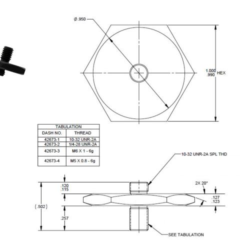
Isolated mounting adapter with 1 inch hex for use with accelerometers with a 10-32 thread.
