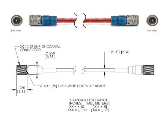
The 3060D cable assembly delivers the highest flexibility along with a wide temperature range. Both ends of the cable are terminated with 10-32 stainless steel connectors and a welded center pin provides maximum pull strength and lowest noise. All critical parameters are 100% tested. The cable capacitance is measured, recorded and the value is provided with each cable assembly.
