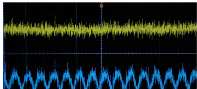
Figure 3: Yellow trace is the transducers noise level before ingress. The blue trace shows the noise level after water ingress.
