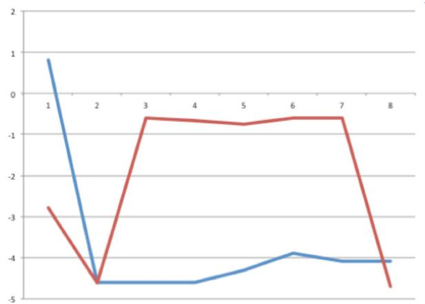
Chart 1: ZMO shift in mV vs. time in days. Red trace is concentrated antifreeze and the blue is tap water. Some of the initial shift is attributed to temperature change.
