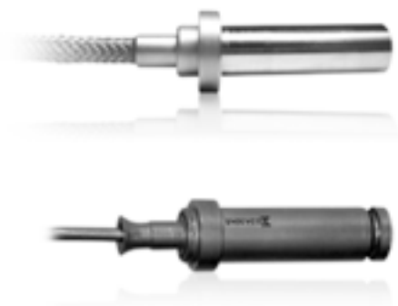
Figure 2: A few examples of Endevco® pressure sensor packages and cables to accommodate a variety of mounting configurations. Both use hardline cable while the top sensor has a protective shield over the cable.
