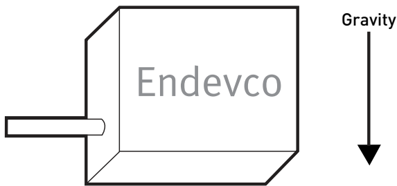
Figure 2 Showing a typical Endevco VC accelerometer on its side. This is the "zero g" position.
