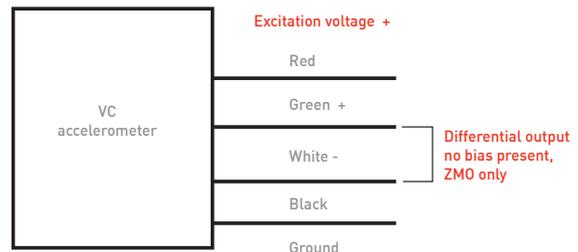
Figure 3 Showing proper connections for a differential output. The green and white wires connect to a differential amplifier.
