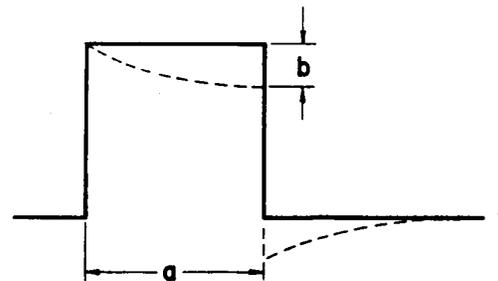
Figure 3-15 Theoretical responses from accelerometers exposed to long-duration square wave shock motions.
