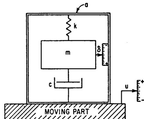
Figure 3-1 Single-degree-of-freedom seismic accelerometer consisting of a mass element  $M$  supported by spring  $K$  with damping  $C$ . The case of the accelerometer is attached to the moving part whose motion is to be measured.
