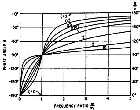
Figure 3-3 Phase angle response of seismic accelerometer indicates the relative displacement,  $\delta$ , to the applied acceleration,  $\ddot{u}$ .
