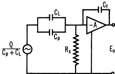
Figure 3-5 Simplified diagram of a charge amplifier.
