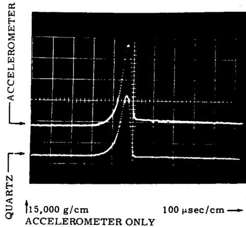
Figure 3-18 Accelerometer shows positive zero shift at 60,000 g.
