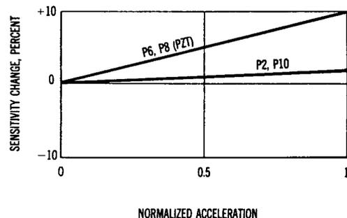
Figure 3-8 Amplitude linearity characteristic of piezoelectric accelerometers shows the sensitivity increasing with acceleration.
