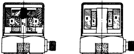
Figure 3-4 Piezoelectric accelerometers showing the compression and shear type constructions.
