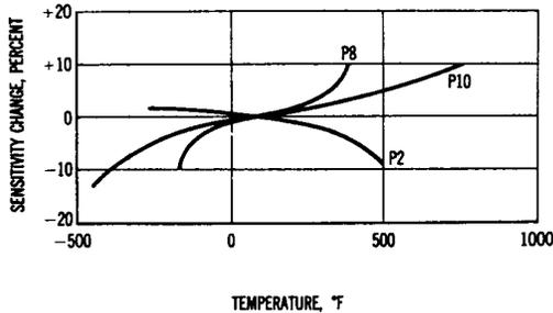
Figure 3-9 Typical temperature response characteristics show charge sensitivity changes for accelerometers using different crystal materials.
