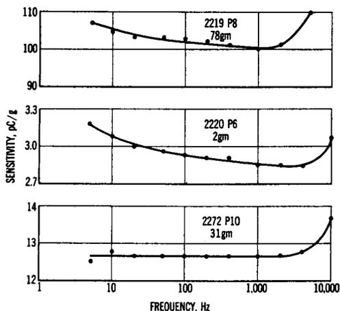
Figure 3-6 Charge frequency response characteristics of piezoelectric accelerometers representing various accelerometer designs and crystal materials.
