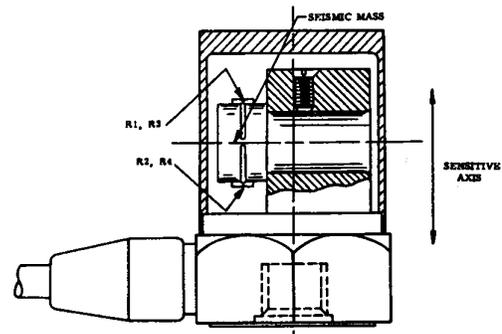
Figure 3-12 Sketch of a piezoresistive strain gage accelerometer.
