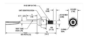
STANDARD TOLERANCE INCHES (MILLIMETERS) .XX = +/- .03 (.X = +/- .8) .XXX = +/- .010 (.XX = +/- .25)
