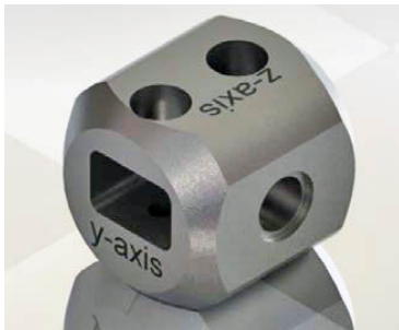
Figure 6: Triaxial calibration fixture used on the 7274.
