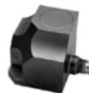
This model 63C12/63C13 Triaxial accelerometer is electrically isolated, hermetically sealed, and has a sensitivity of 1000 mV/g (C13) and 100 mV/g (C12) respectively. Frequency response is 0.5 Hz-3 kHz ( $\pm 5\%$ ).
