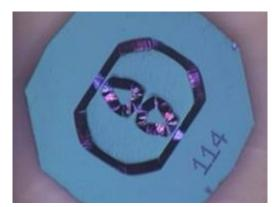
Figure 1 – Photograph of diaphragm taken with scanning electron microscope 0.05 in. (1.25 mm) O.D.
