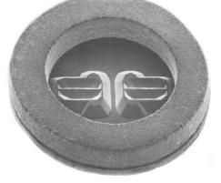
Figure 3 – Photograph of diaphragm, glass-bonded to heavy silicon ring, 0.1 in (2.5 mm) O.D> by 0.02 in (0.5 mm) thick.
