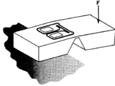
Figure 2: Transverse gage on etched bar
