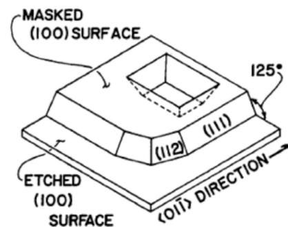
Figure 1: Anisotropic etch patterns in silicon
