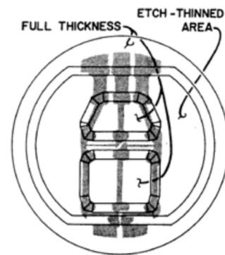
Figure 3: Pressure transducer die
