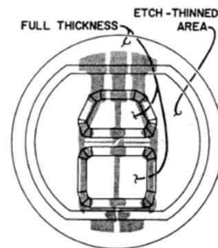
Figure 3: Pressure transducer die
