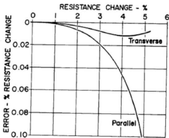
Figure 6: Non-linearity of a half-bridge pair
