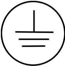
Protective conductor terminal. For protection against electrical shock in case of a fault. Used with field wiring terminals to indicate the terminal which must be connected to ground before operating the equipment.
